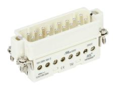
METE male insert, connector housing size 16A, 16-pole, screw terminals, accepts wire size 18-14 AWG, 16 amp, 600 VAC/VDC, poles numbered 1 to 16. For use with METE multi-wire housings.
