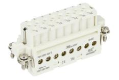
METE female insert, connector housing size 16A, 16-pole, screw terminals, accepts wire size 18-14 AWG, 16 amp, 600 VAC/VDC, poles numbered 1 to 16. For use with METE multi-wire housings.
