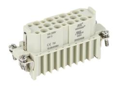
METE female insert, connector housing size 16A, 25-pole, crimped contact, 10 amp, 600 VAC/VDC, poles numbered 1 to 25. For use with METE multi-wire housings. Requires 10 amp female contacts METE 14103xxx.
