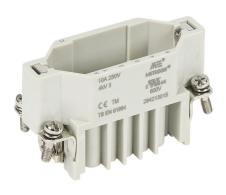
METE male insert, connector housing size 10A, 15-pole, crimped contact, 10 amp, 600 VAC/VDC, poles numbered 1 to 15. For use with METE multi-wire housings. Requires 10 amp male contacts METE 14104xxx.
