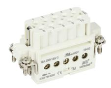
METE female insert, connector housing size 10A, 10-pole, screw terminals, accepts wire size 18-14 AWG, 16 amp, 600 VAC/VDC, poles numbered 1 to 10. For use with METE multi-wire housings.
