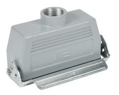
METE coupler housing, single lever, top entry, connector housing size 24B, (1) 3/4 NPT threaded hole, heavy-duty die cast aluminum. For use with METE size 24B 2-peg connector housings.
