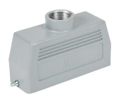
METE hood housing, 2-peg, top entry, connector housing size 24B, (1) 3/4 NPT threaded hole, heavy-duty die cast aluminum. For use with METE size 24B single lever connector housings.
