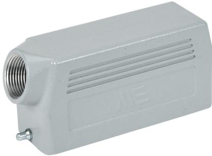
METE hood housing, 2-peg, side entry, connector housing size 24B, (1) 3/4 NPT threaded hole, heavy-duty die cast aluminum. For use with METE size 24B single lever connector housings.
