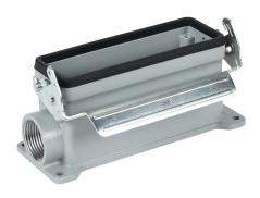
METE surface mount housing, single lever, side entry, connector housing size 24B, (1) 3/4 NPT threaded hole, heavy-duty die cast aluminum. For use with METE size 24B 2-peg connector housings.
