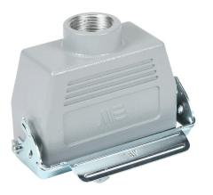
METE coupler housing, single lever, top entry, connector housing size 16B, (1) 3/4 NPT threaded hole, heavy-duty die cast aluminum. For use with METE size 16B 2-peg connector housings.
