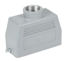
METE hood housing, 2-peg, top entry, connector housing size 16B, (1) 3/4 NPT threaded hole, heavy-duty die cast aluminum. For use with METE size 16B single lever connector housings.
