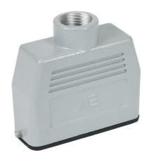
METE hood housing, 2-peg, top entry, connector housing size 16A, (1) 1/2 NPT threaded hole, heavy-duty die cast aluminum. For use with METE size 16A single lever connector housings.
