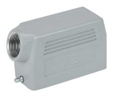
METE hood housing, 2-peg, side entry, connector housing size 16B, (1) 3/4 NPT threaded hole, heavy-duty die cast aluminum. For use with METE size 16B single lever connector housings.
