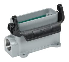
METE surface mount housing, single lever, side entry, connector housing size 16A, (1) 1/2 NPT threaded hole, heavy-duty die cast aluminum. For use with METE size 16A 2-peg connector housings.
