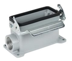
METE surface mount housing, single lever, side entry, connector housing size 16B, (1) 3/4 NPT threaded hole, heavy-duty die cast aluminum. For use with METE size 16B 2-peg connector housings.
