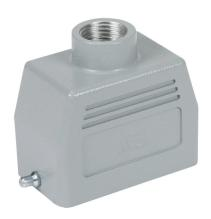
METE hood housing, 2-peg, top entry, connector housing size 10B, (1) 1/2 NPT threaded hole, heavy-duty die cast aluminum. For use with METE size 10B single lever connector housings.
