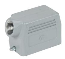
METE hood housing, 2-peg, side entry, connector housing size 10B, (1) 1/2 NPT threaded hole, heavy-duty die cast aluminum. For use with METE size 10B single lever connector housings.
