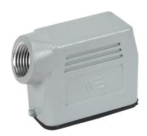
METE hood housing, 2-peg, side entry, connector housing size 10A, (1) 1/2 NPT threaded hole, heavy-duty die cast aluminum. For use with METE size 10A single lever connector housings.
