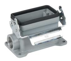
METE surface mount housing, single lever, side entry, connector housing size 10B, (1) 1/2 NPT threaded hole, heavy-duty die cast aluminum. For use with METE size 10B 2-peg connector housings.
