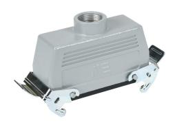
METE coupler housing, double lever, top entry, connector housing size 24B, (1) 3/4 NPT threaded hole, heavy-duty die cast aluminum. For use with METE size 24B 4-peg connector housings.
