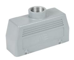
METE hood housing, 4-peg, top entry, connector housing size 24B, (1) 3/4 NPT threaded hole, heavy-duty die cast aluminum. For use with METE size 24B double lever connector housings.
