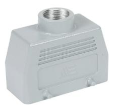
METE hood housing, 4-peg, top entry, connector housing size 16B, (1) 3/4 NPT threaded hole, heavy-duty die cast aluminum. For use with METE size 16B double lever connector housings.
