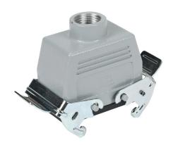
METE coupler housing, double lever, top entry, connector housing size 10B, (1) 1/2 NPT threaded hole, heavy-duty die cast aluminum. For use with METE size 10B 4-peg connector housings.
