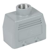
METE hood housing, 4-peg, top entry, connector housing size 10B, (1) 1/2 NPT threaded hole, heavy-duty die cast aluminum. For use with METE size 10B double lever connector housings.
