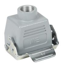
METE coupler housing, single lever, top entry, connector housing size 6B, (1) 1/2 NPT threaded hole, heavy-duty die cast aluminum. For use with METE size 6B 2-peg connector housings.
