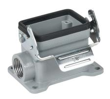
METE surface mount housing, single lever, side entry, connector housing size 6B, (1) 1/2 NPT threaded hole, heavy-duty die cast aluminum. For use with METE size 6B 2-peg connector housings.
