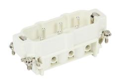
METE male insert, connector housing size 16B, 6-pole, screw terminals, accepts wire size 11 AWG, 35 amp, 600 VAC/VDC, poles numbered 1 to 6. For use with METE multi-wire housings.
