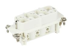
METE female insert, connector housing size 16B, 6-pole, screw terminals, accepts wire size 10 AWG, 35 amp, 600 VAC/VDC, poles numbered 1 to 6. For use with METE multi-wire housings.
