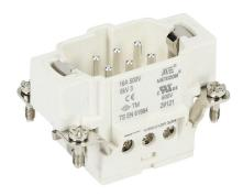
METE male insert, connector housing size 6B, 6-pole, screw terminals, accepts wire size 18-14 AWG, 16 amp, 600 VAC/VDC, poles numbered 1 to 6. For use with METE multi-wire housings.
