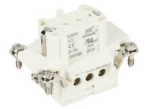
METE female insert, connector housing size 6B, 6-pole, screw terminals, accepts wire size 18-14 AWG, 16 amp, 600 VAC/VDC, poles numbered 1 to 6. For use with METE multi-wire housings.
