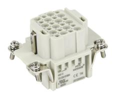
METE female insert, connector housing size 6B, 24-pole, crimped contact, 10 amp, 600 VAC/VDC, poles numbered 1 to 24. For use with METE multi-wire housings. Requires 10 amp female contacts METE 14103xxx.
