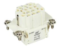
METE female insert, connector housing size 6B, 10-pole, crimped contact, 16 amp, 600 VAC/VDC, poles numbered 1 to 10. For use with METE multi-wire housings. Requires 16 amp female contacts METE 14105xxx.
