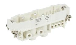
METE male insert, connector housing size 24B, 12-pole, screw terminals, accepts wire size 6-16 AWG, 26-14 AWG, 80 amp (4-pole), 16 amp (8-pole), 600 VAC/VDC, poles numbered 1 to 12. For use with METE multi-wire housings.
