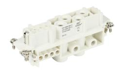
METE female insert, connector housing size 24B, 12-pole, screw terminals, accepts wire size 6-16 AWG, 26-14 AWG, 80 amp (4-pole), 16 amp (8-pole), 600 VAC/VDC, poles numbered 1 to 12. For use with METE multi-wire housings.
