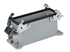
METE surface mount housing, double lever, side entry, connector housing size 24B, (1) 3/4 NPT threaded hole, heavy-duty die cast aluminum. For use with METE size 24B 4-peg connector housings.
