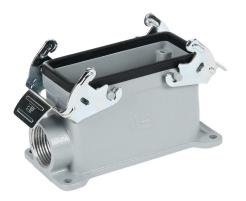
METE surface mount housing, double lever, side entry, connector housing size 16B, (1) 3/4 NPT threaded hole, heavy-duty die cast aluminum. For use with METE size 16B 4-peg connector housings.
