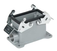
METE surface mount housing, double lever, side entry, connector housing size 10B, (1) 1/2 NPT threaded hole, heavy-duty die cast aluminum. For use with METE size 10B 4-peg connector housings.
