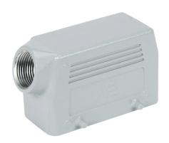
METE hood housing, 4-peg, side entry, connector housing size 16B, (1) 3/4 NPT threaded hole, heavy-duty die cast aluminum. For use with METE size 16B double lever connector housings.
