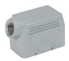
METE hood housing, 4-peg, side entry, connector housing size 10B, (1) 1/2 NPT threaded hole, heavy-duty die cast aluminum. For use with METE size 10B double lever connector housings.
