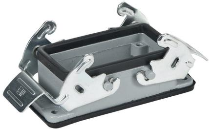
METE bulkhead housing, double lever, connector housing size 10B, heavy-duty die cast aluminum. For use with METE size 10B 4-peg connector housings.
