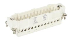
METE male insert, connector housing size 24B, 24-pole, screw terminals, accepts wire size 18-14 AWG, 16 amp, 600 VAC/VDC, poles numbered 1 to 24. For use with METE multi-wire housings.
