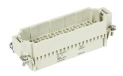
METE male insert, connector housing size 24B, 108-pole, crimped contact, 10 amp, 600 VAC/VDC, poles numbered 1 to 108. For use with METE multi-wire housings. Requires 10 amp male contacts METE 14104xxx.
