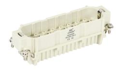
METE male insert, connector housing size 24B, 64-pole, crimped contact, 10 amp, 600 VAC/VDC, poles numbered 1 to 64. For use with METE multi-wire housings. Requires 10 amp male contacts METE 14104xxx.
