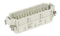
METE male insert, connector housing size 24B, 46-pole, crimped contact, 16 amp, 600 VAC/VDC, poles numbered 1 to 46. For use with METE multi-wire housings. Requires 16 amp male contacts METE 14106xxx.
