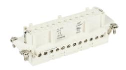
METE female insert, connector housing size 24B, 24-pole, screw terminals, accepts wire size 18-14 AWG, 16 amp, 600 VAC/VDC, poles numbered 1 to 24. For use with METE multi-wire housings.
