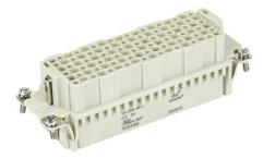
METE female insert, connector housing size 24B, 108-pole, crimped contact, 10 amp, 600 VAC/VDC, poles numbered 1 to 108. For use with METE multi-wire housings. Requires 10 amp female contacts METE 14103xxx.
