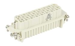
METE female insert, connector housing size 24B, 64-pole, crimped contact, 10 amp, 600 VAC/VDC, poles numbered 1 to 64. For use with METE multi-wire housings. Requires 10 amp female contacts METE 14103xxx.
