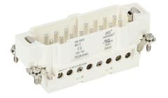
METE male insert, connector housing size 16B, 16-pole, screw terminals, accepts wire size 18-14 AWG, 16 amp, 600 VAC/VDC, poles numbered 1 to 16. For use with METE multi-wire housings.
