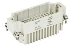
METE male insert, connector housing size 16B, 72-pole, crimped contact, 10 amp, 600 VAC/VDC, poles numbered 1 to 72. For use with METE multi-wire housings. Requires 10 amp male contacts METE 14104xxx.
