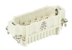
METE male insert, connector housing size 16B, 40-pole, crimped contact, 10 amp, 600 VAC/VDC, poles numbered 1 to 40. For use with METE multi-wire housings. Requires 10 amp male contacts METE 14104xxx.
